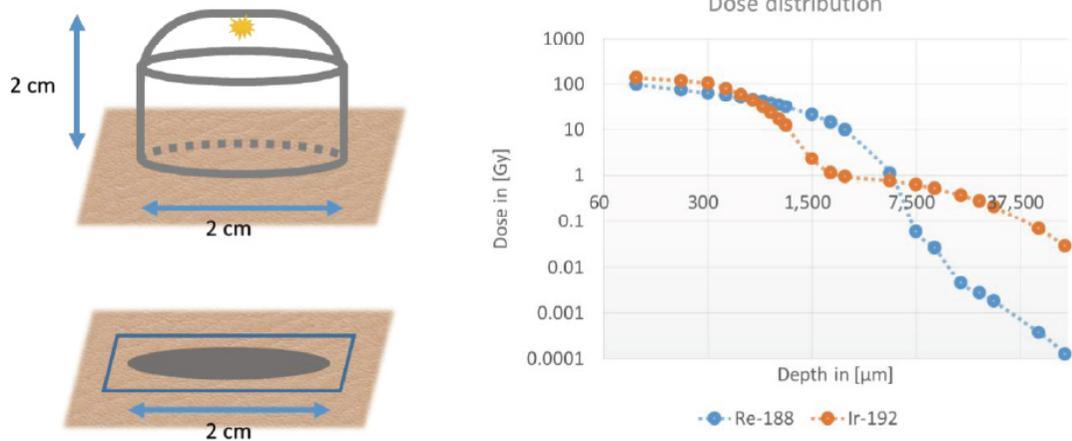
**Figure 1:** Right, dose at different skin depth for Rhenium-188 versus Iridium-192 for a comparable total dose of 65 Gy within the first 1.5mm. Simulations were performed using NRC’s VARSKIN 5.2 software [14]. Left, schematics of simulated scenarios with VARSKIN.
